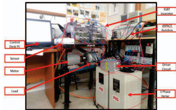
Fig. 5. Experimental rig of the IM electrical drive where the combined estimator approach is applied
